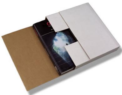
**One Piece Folders:** OPF's are containers which wrap around a product and provide a flat bottom surface and used to package shallow depth items such as book-shaped objects and pictures. Usually manufactured with white board. The One Piece Folder has a flat bottom with two short flaps forming the sides at each end and two longer, wider flaps that form the front, back and top of the box. The wider flaps either meet or overlap
