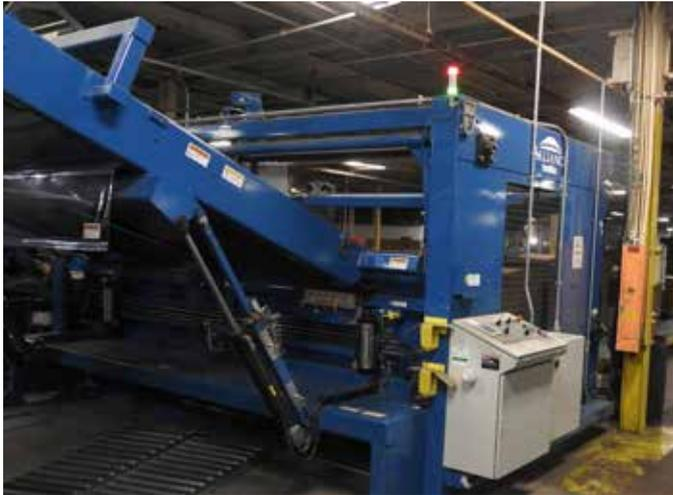
**Two flexos in Akers Packaging's Chicago plant are equipped with Alliance prefeeders.**
