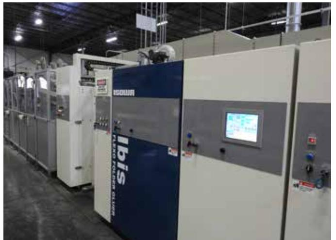
**An Isowa Ibis, a 47-inch by 120-inch flexo folder gluer complements the Isowa Falcon at Akers' Middletown, Ohio, plant.**
