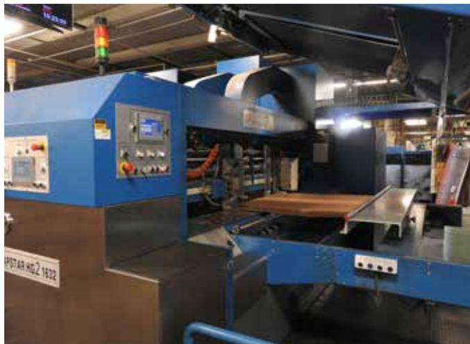
**A 3-color Apstar flexo folder gluer from Haire Group has a die cut section and adds capacity to Akers production lines.**
